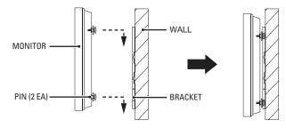
Figure 4. Attaching Monitor to Wall
